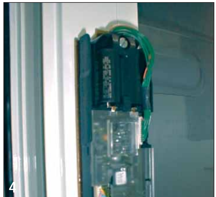
Insert battery and secure with clamp.
