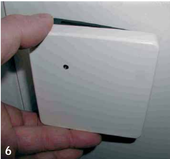
6 Snap on the in-wall socket cover ES5410 so that the viewer is on the upper left and the LED is visible through the viewer.
