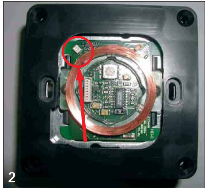
2 The LED positioned in the upper left. Screw holes aligned horizontally or vertically with the in-wall socket.
