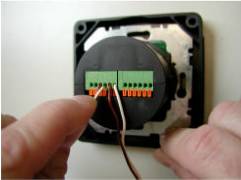
4. Install all necessary connections (power supply, relay, etc.) as shown in the wiring plan beyond. Plug the still connection cables into the right connector. They fit automatically.
