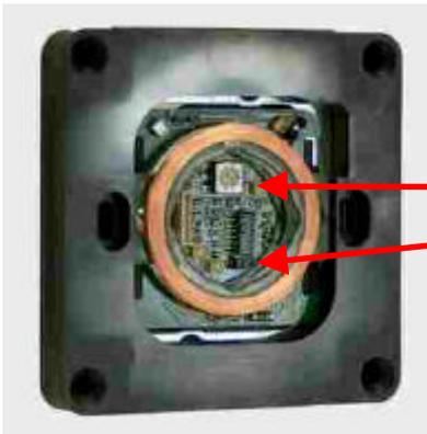
5. Mount the wallreader onto the socket using the enclosed screws. Turn the screws carefully so that the circuit board doesn't become distorted. Alternative use four screws in the edges. Check the adress switch and the termination switch (on/off).
