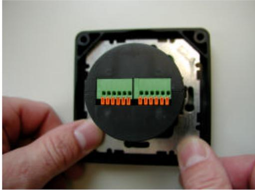
1. Lock the reading-module ES5401 in backside of the cover ES5410.
